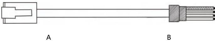
Figure 4.9 The Communication Cable Of Servo Drive With PLC
